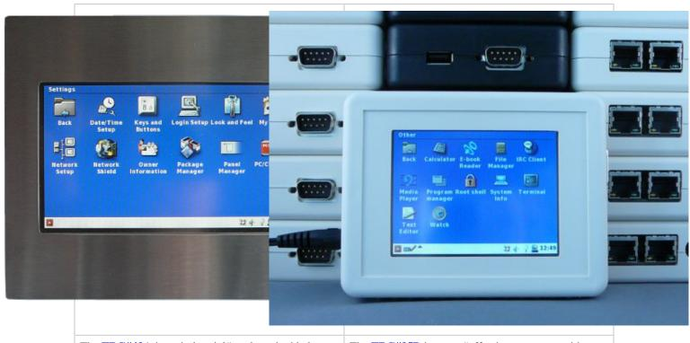
The <u>TPC#43A</u> is an industrial#grade embedded computer with a **Color, TFT LCD and Touch panel** targeting Building Automation applications.
