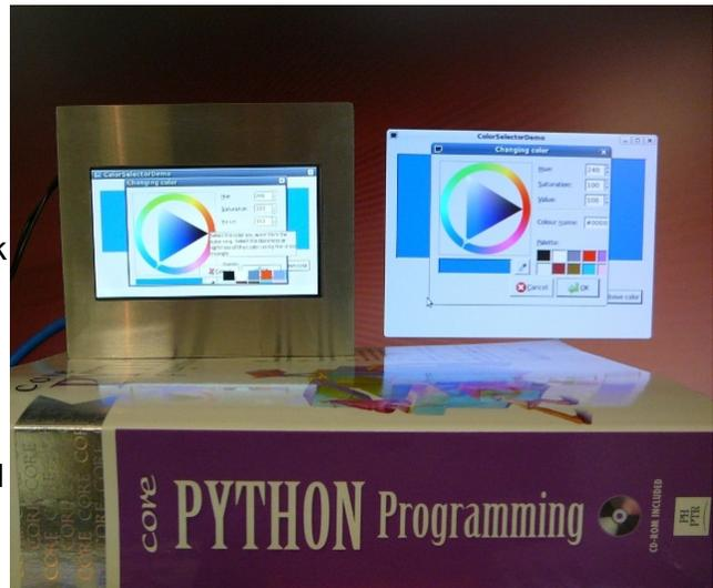
Techsol's Medallion Touch Panel Computers (TPCs) provide just this Linux GTK target. Loaded with one of our GPE ([gpe.handhelds.org](http://gpe.handhelds.org)) images, the TPC provides a full Linux environment running a GTK GUI on an X (X11) server. Just like your [Linux desktop](#).
